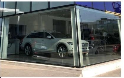
Tempered glass undergoes a specialized heat treatment process that imparts exceptional strength and durability. When broken, tempered glass fractures into small, blunt pieces rather than sharp shards, reducing the risk of injury. This type of security glass is particularly suitable for applications where resistance to impact is crucial. Example: SECURIT®
